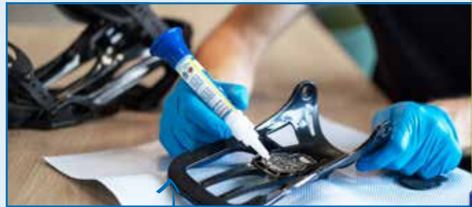
Bonding of a snowboard binding
